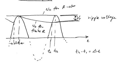
Diode conducts from to to tr. -> capacitor is charged after t2, the capacitor discharges.
