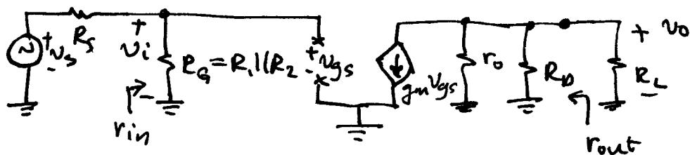
$$r_{in} = R_g = R_1 \parallel R_2$$
