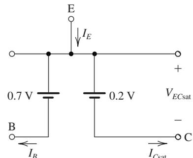
$$|V_{CEsat}| = V_T \ln \left[ \frac{1 + (\beta_{forced} + 1)/\beta_F}{1 - \beta_{forced}/\beta_F} \right]$$
