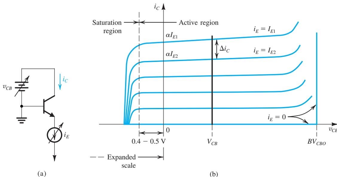
**FIGURE 5.18** The  $i_C$ - $v_{CB}$  characteristics for an  $n\text{pn}$  transistor.
