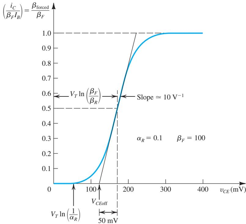
**FIGURE 5.25** Plot of the normalized  $i_C$  versus  $v_{CE}$  for an  $npn$  transistor with  $\beta_F = 100$  and  $\alpha_R = 0.1$ . This is a plot of Eq. (5.47), which is derived using the Ebers-Moll model.
