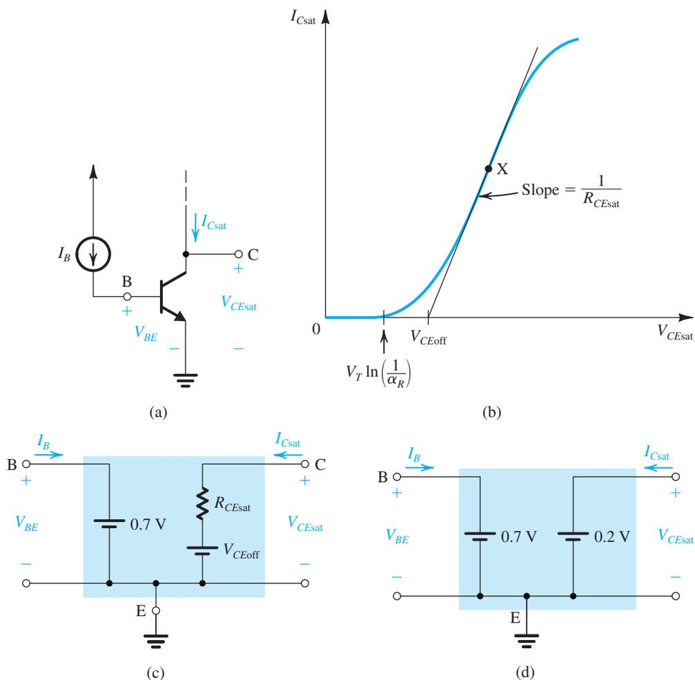
**FIGURE 5.24** (a) An npn transistor operated in saturation mode with a constant base current  $I_B$ . (b) The  $i_C-v_{CE}$  characteristic curve corresponding to  $i_B = I_B$ . The curve can be approximated by a straight line of slope  $1/R_{CEsat}$ . (c) Equivalent-circuit representation of the saturated transistor. (d) A simplified equivalent-circuit model of the saturated transistor.
