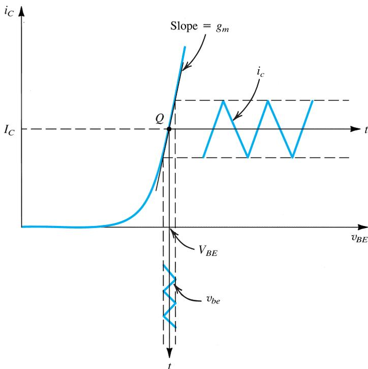
**FIGURE 5.49** Linear operation of the transistor under the small-signal condition: A small signal  $v_{be}$  with a triangular waveform is superimposed on the dc voltage  $V_{BE}$ . It gives rise to a collector signal current  $i_c$ , also of triangular waveform, superimposed on the dc current  $I_C$ .  $i_c = g_m v_{be}$ , where  $g_m$  is the slope of the  $i_C$ - $v_{BE}$  curve at the bias point  $Q$ .
