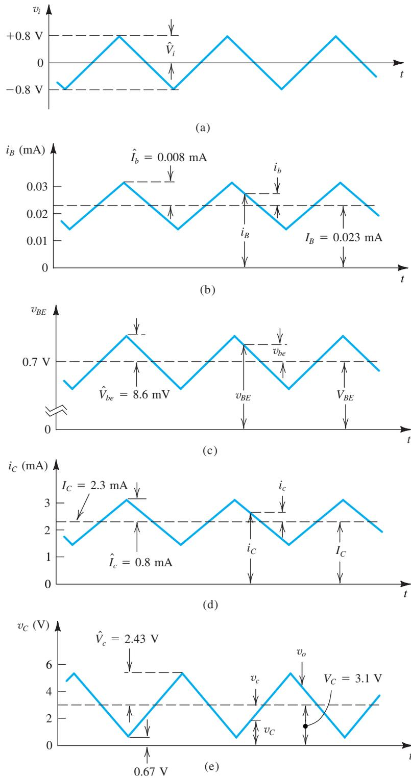
FIGURE 5.54 Signal waveforms in the circuit of Fig. 5.53.
