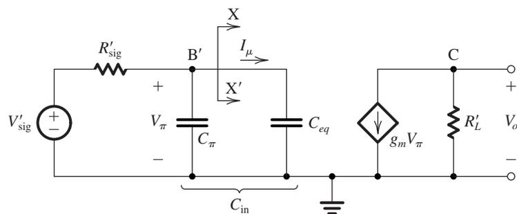
$$C_{\text{in}} = C_{\pi} + C_{\text{eq}} \\ = C_{\pi} + C_{\mu}(1 + g_m R'_L)$$
