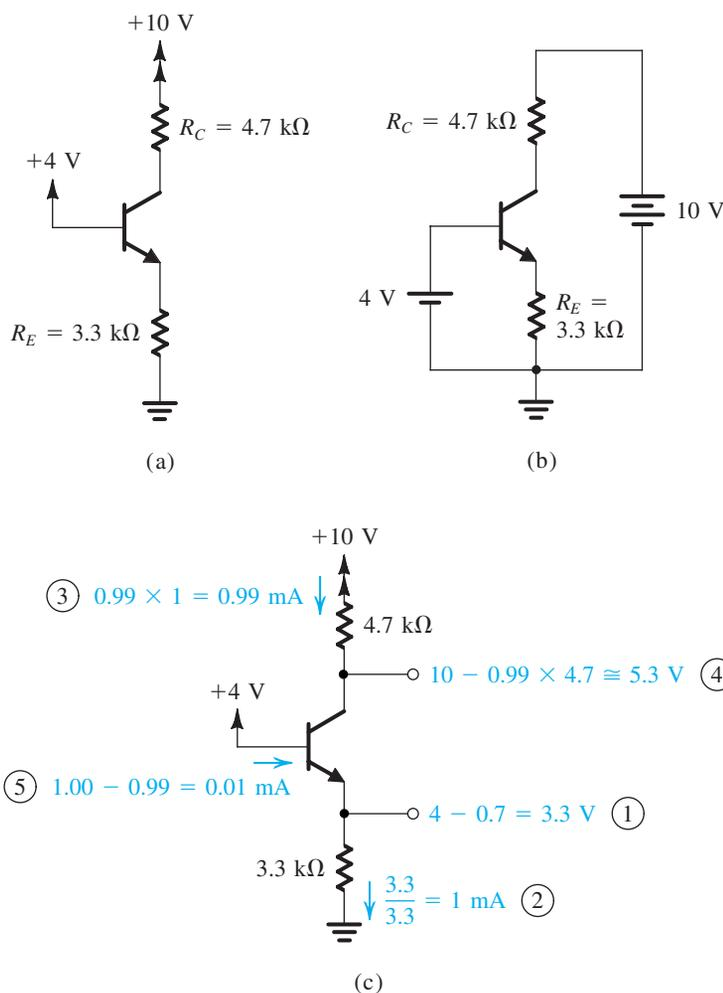
**FIGURE 5.34** Analysis of the circuit for Example 5.4: (a) circuit; (b) circuit redrawn to remind the reader of the convention used in this book to show connections to the power supply; (c) analysis with the steps numbered.
