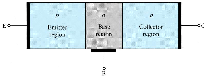
**FIGURE 5.2** A simplified structure of the *pnp* transistor.
