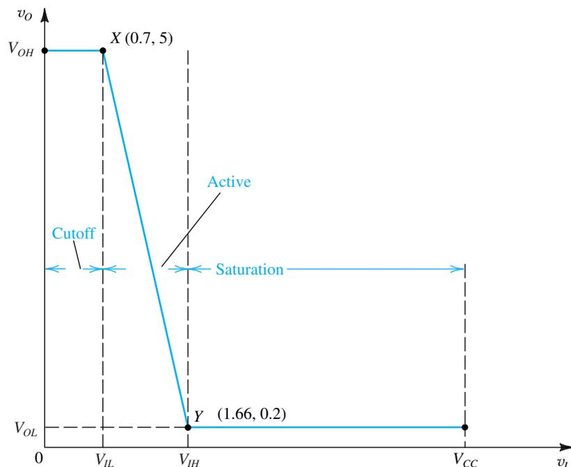
**FIGURE 5.75** Sketch of the voltage transfer characteristic of the inverter circuit of Fig. 5.74 for the case  $R_B = 10$  k $\Omega$ ,  $R_C = 1$  k $\Omega$ ,  $\beta = 50$ , and  $V_{CC} = 5$  V. For the calculation of the coordinates of X and Y, refer to the text.
