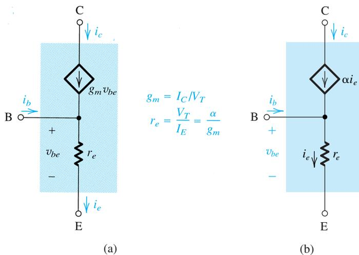
**FIGURE 5.52** Two slightly different versions of what is known as the *T model* of the BJT. The circuit in (a) is a voltage-controlled current source representation and that in (b) is a current-controlled current source representation. These models explicitly show the emitter resistance  $r_e$  rather than the base resistance  $r_\pi$  featured in the hybrid- $\pi$  model.
