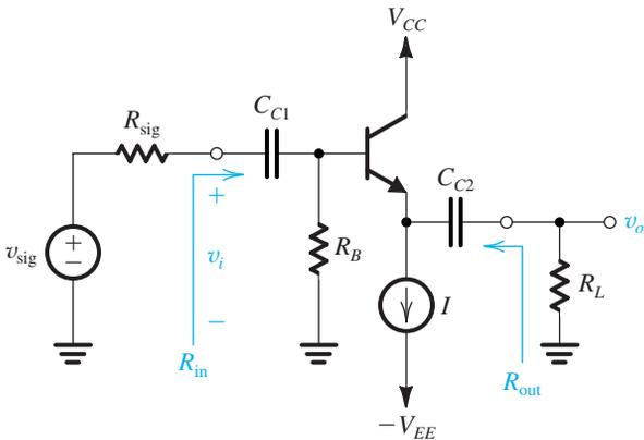
$$R_{in} = R_B \parallel (\beta + 1)[r_e + (r_o \parallel R_L)]$$
