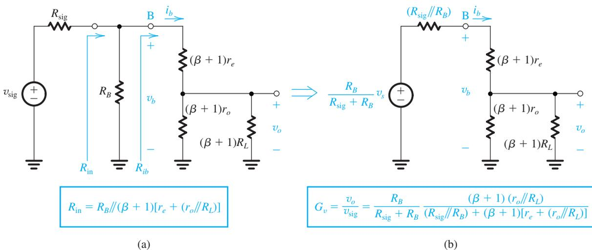
**FIGURE 5.64** (a) An equivalent circuit of the emitter follower obtained from the circuit in Fig. 5.63(c) by reflecting all resistances in the emitter to the base side. (b) The circuit in (a) after application of the Thévenin theorem to the input circuit composed of  $V_{sig}$ ,  $R_{sig}$ , and  $R_B$ .
