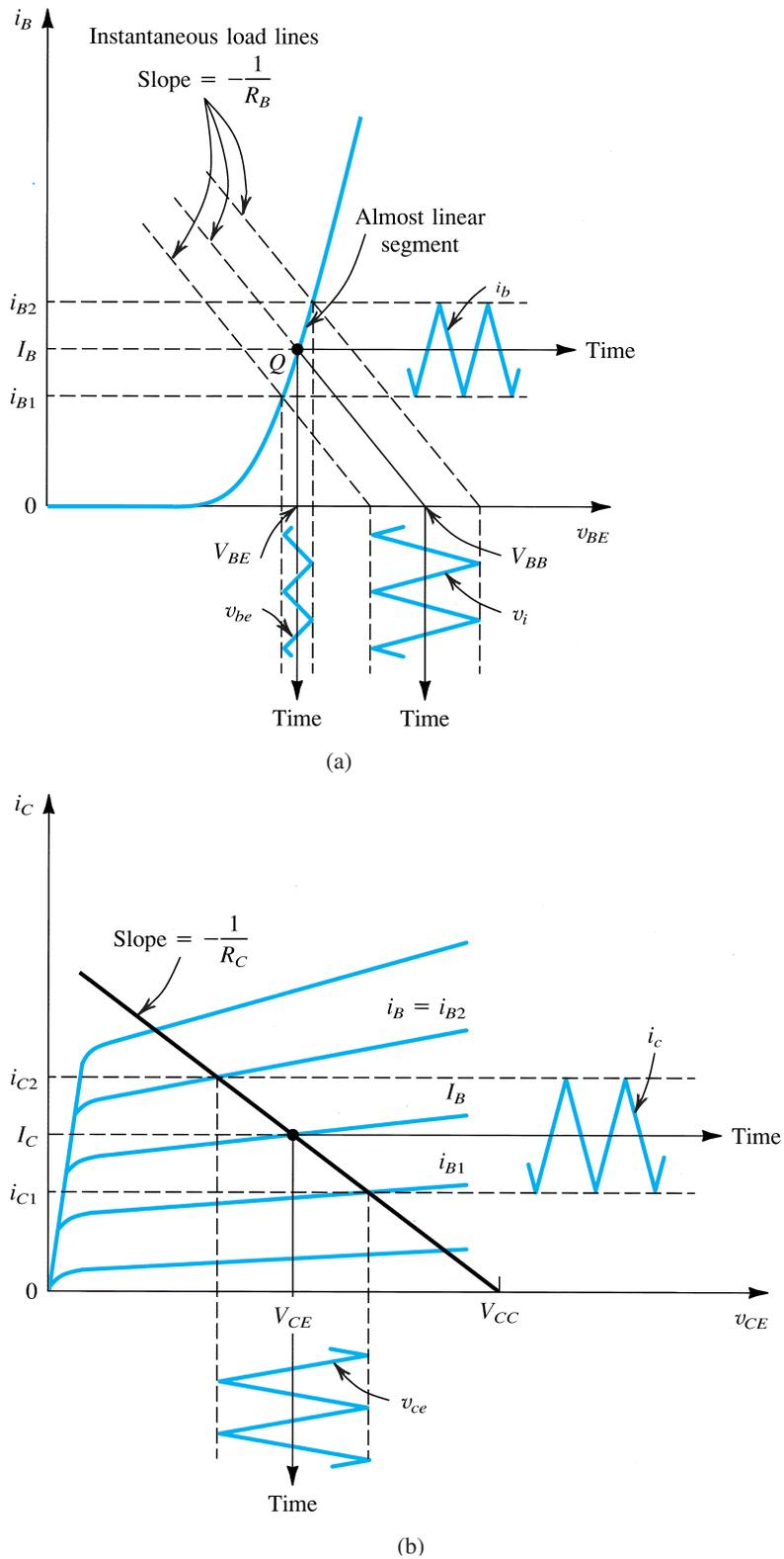
**FIGURE 5.30** Graphical determination of the signal components  $v_{be}$ ,  $i_b$ ,  $i_c$ , and  $v_{ce}$  when a signal component  $v_i$  is superimposed on the dc voltage  $V_{BE}$  (see Fig. 5.27).
