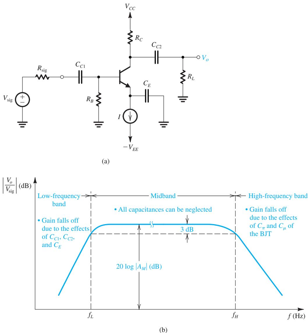
**FIGURE 5.71** (a) Capacitively coupled common-emitter amplifier. (b) Sketch of the magnitude of the gain of the CE amplifier versus frequency. The graph delineates the three frequency bands relevant to frequency response determination.
