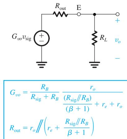
**FIGURE 5.66** Thévenin equivalent circuit of the output of the emitter follower of Fig. 5.63(a). This circuit can be used to find  $v_o$  and hence the overall voltage gain  $v_o/v_s$  for any desired  $R_L$ .
