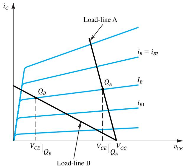
**FIGURE 5.31** Effect of bias-point location on allowable signal swing: Load-line A results in bias point  $Q_A$  with a corresponding  $V_{CE}$  which is too close to  $V_{CC}$  and thus limits the positive swing of  $v_{CE}$ . At the other extreme, load-line B results in an operating point too close to the saturation region, thus limiting the negative swing of  $v_{CE}$ .
