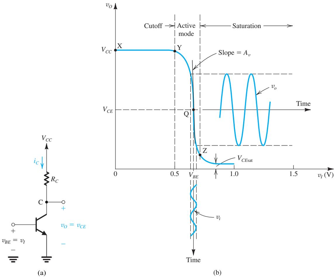
**FIGURE 5.26** (a) Basic common-emitter amplifier circuit. (b) Transfer characteristic of the circuit in (a). The amplifier is biased at a point Q, and a small voltage signal  $v_i$  is superimposed on the dc bias voltage  $V_{BE}$ . The resulting output signal  $v_o$  appears superimposed on the dc collector voltage  $V_{CE}$ . The amplitude of  $v_o$  is larger than that of  $v_i$  by the voltage gain  $A_v$ .
