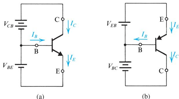
FIGURE 5.14 Voltage polarities and current flow in transistors biased in the active mode.
