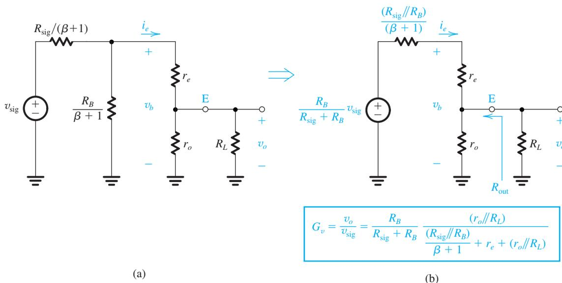
**FIGURE 5.65** (a) An alternate equivalent circuit of the emitter follower obtained by reflecting all base-circuit resistances to the emitter side. (b) The circuit in (a) after application of the Thévenin theorem to the input circuit composed of  $V_{\text{sig}}$ ,  $R_{\text{sig}}/(\beta + 1)$ , and  $R_B/(\beta + 1)$ .
