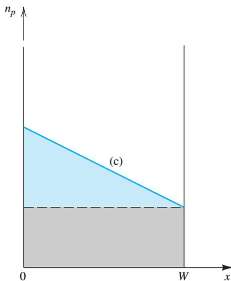
**FIGURE 5.76** The minority-carrier charge stored in the base of a saturated transistor can be divided into two components: That in blue produces the gradient that gives rise to the diffusion current across the base, and that in gray results in driving the transistor deeper into saturation.
