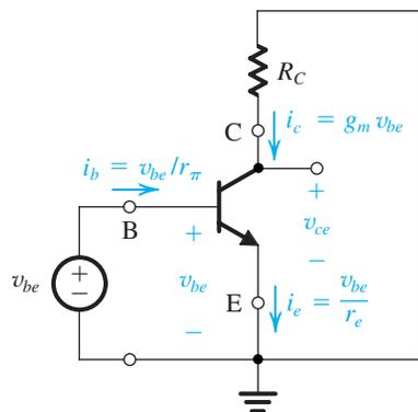
**FIGURE 5.50** The amplifier circuit of Fig. 5.48(a) with the dc sources  $V_{BE}$  and  $V_{CC}$  eliminated (short circuited). Thus only the signal components are present. Note that this is a representation of the signal operation of the BJT and not an actual amplifier circuit.
