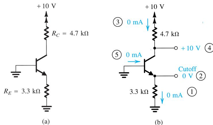
**FIGURE 5.36** Example 5.6: (a) circuit; (b) analysis with the order of the analysis steps indicated by circled numbers.
