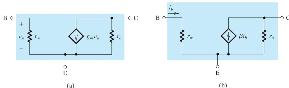
**FIGURE 5.58** The hybrid- $\pi$  small-signal model, in its two versions, with the resistance  $r_o$  included.
