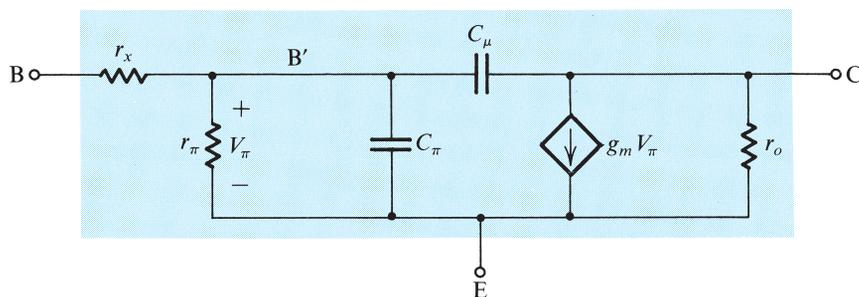
FIGURE 5.67 The high-frequency hybrid- $\pi$  model.
