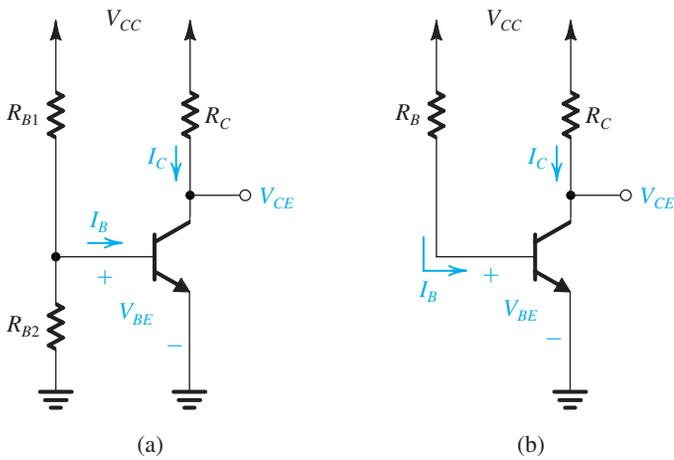
**FIGURE 5.43** Two obvious schemes for biasing the BJT: (a) by fixing  $V_{BE}$ ; (b) by fixing  $I_B$ . Both result in wide variations in  $I_C$  and hence in  $V_{CE}$  and therefore are considered to be “bad.” Neither scheme is recommended.
