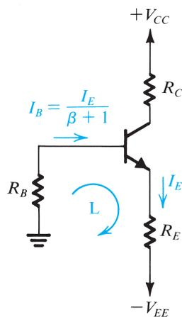
**FIGURE 5.45** Biasing the BJT using two power supplies. Resistor  $R_B$  is needed only if the signal is to be coupled to the base. Otherwise, the base can be connected directly to ground, resulting in almost total independence of the bias current with regard to the value of  $\beta$ .
