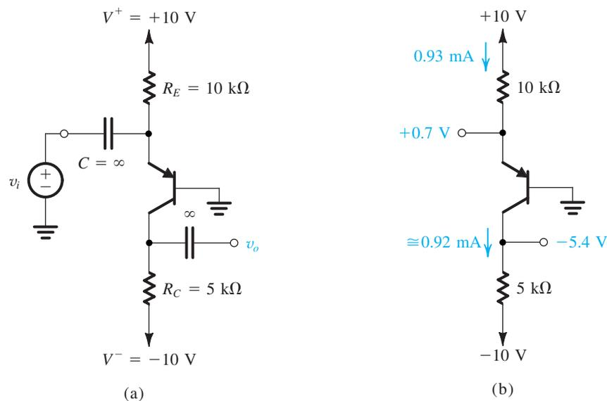
FIGURE 5.55 Example 5.16: (a) circuit; (b) dc analysis;
