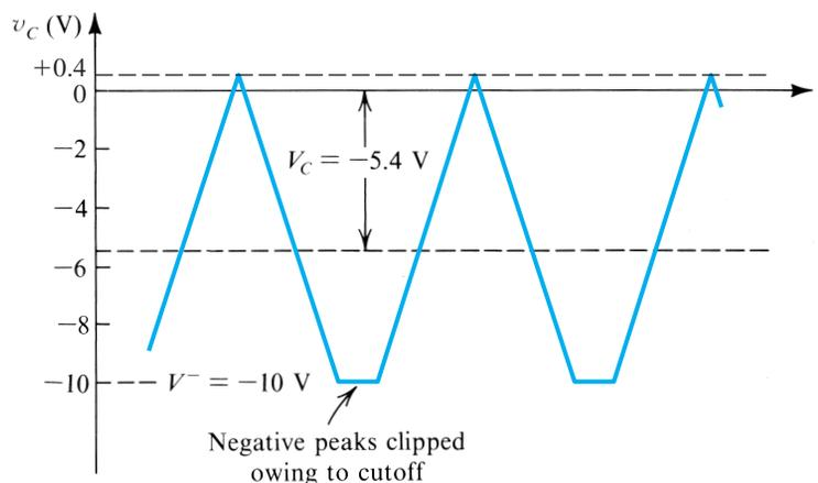
**FIGURE 5.56** Distortion in output signal due to transistor cutoff. Note that it is assumed that no distortion due to transistor nonlinear characteristics is occurring.
