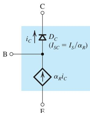
**FIGURE 5.7** Model for the *npn* transistor when operated in the reverse active mode (i.e., with the CBJ forward biased and the EBJ reverse biased).
