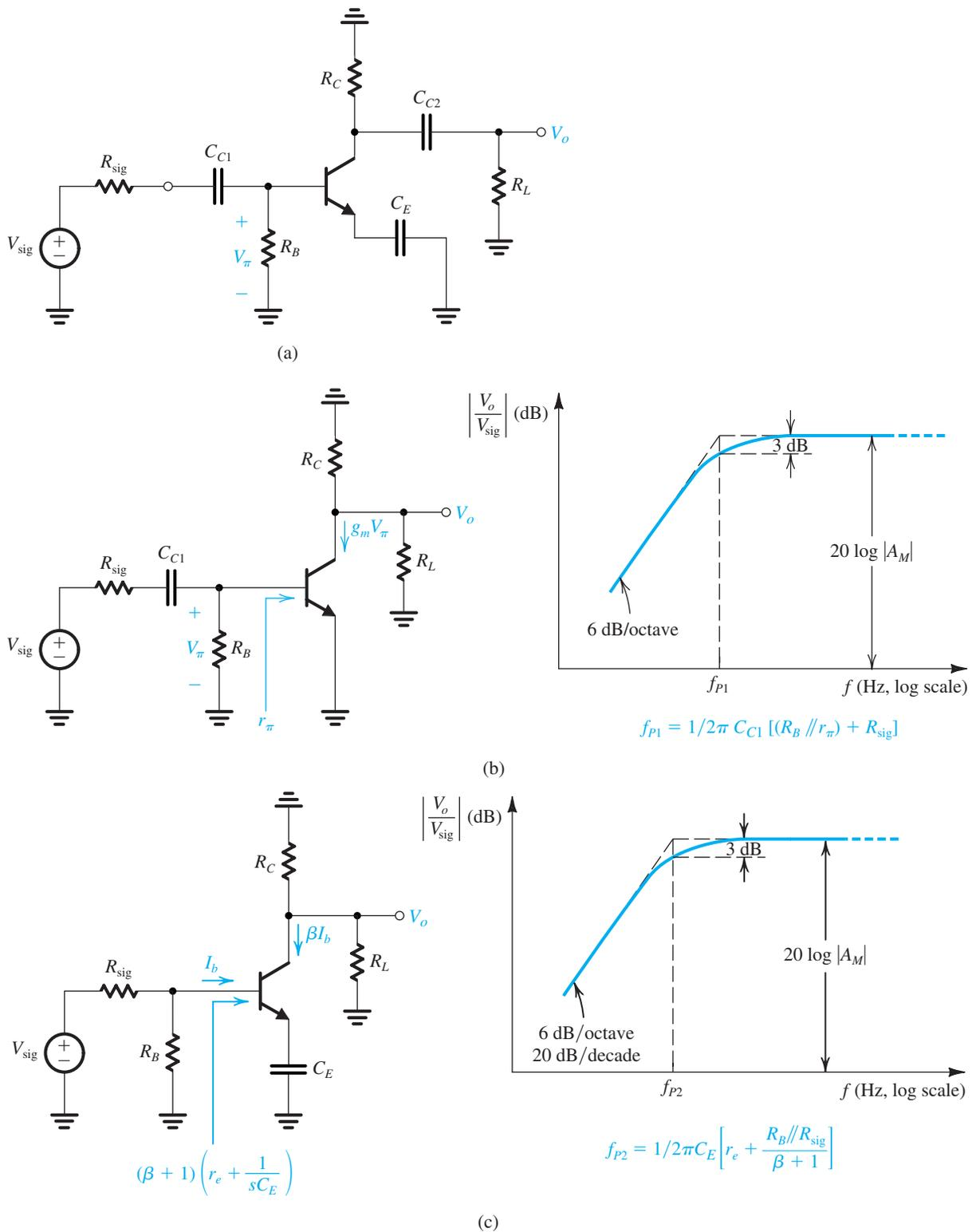
**FIGURE 5.73** Analysis of the low-frequency response of the CE amplifier: (a) amplifier circuits with dc sources removed; (b) the effect of  $C_{C1}$  is determined with  $C_E$  and  $C_{C2}$  assumed to be acting as perfect short circuits; (c) the effect of  $C_E$  is determined with  $C_{C1}$  and  $C_{C2}$  assumed to be acting as perfect short circuits;
