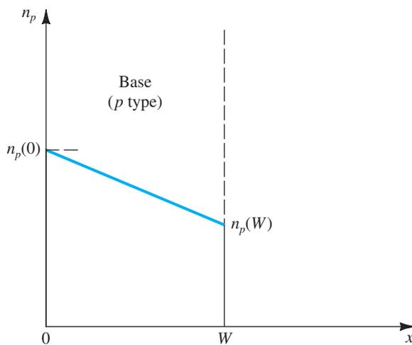
**FIGURE 5.10** Concentration profile of the minority carriers (electrons) in the base of an  $npn$  transistor operating in saturation mode.
