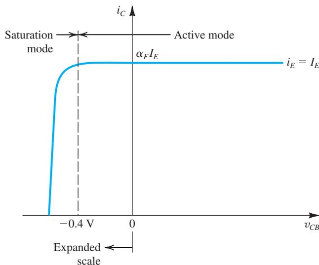
**FIGURE 5.9** The  $i_C$ - $v_{CB}$  characteristics of an  $npn$  transistor fed with a constant emitter current  $I_E$ . The transistor enters the saturation mode of operation for  $v_{CB} < -0.4$  V, and the collector current falls off.
