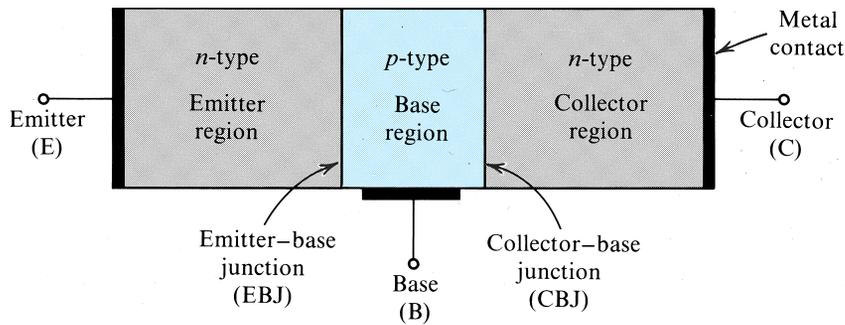
**FIGURE 5.1** A simplified structure of the *npn* transistor.
