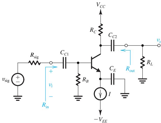
$$R_{in} = R_B \parallel r_{\pi} = R_B \parallel (\beta + 1)r_e$$
