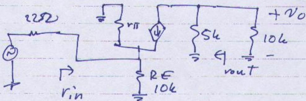
$$r_{ih} = 10k \parallel \frac{r_{\pi}}{\beta + 1} = 10k \parallel \frac{5.53k}{251} = 0.0225 \Omega$$
