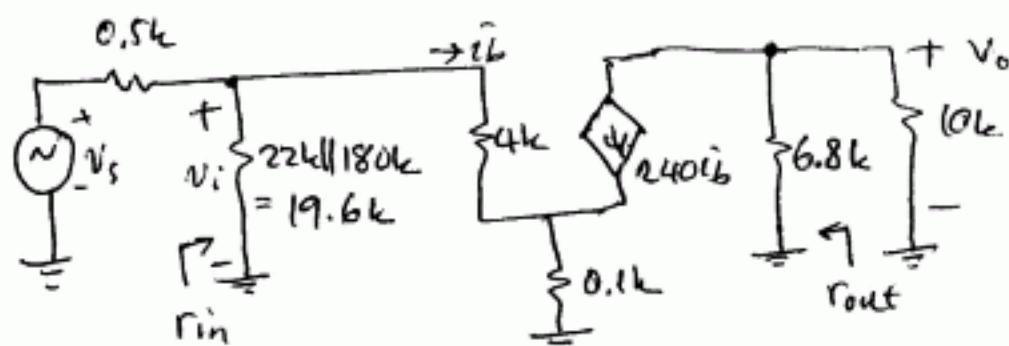
$$r_{in} = 19.6 \text{ k} \parallel [4 \text{ k} + 0.1(240+1)] = 19.6 \text{ k} \parallel 28.1 \text{ k} = 11.54 \text{ k}$$
