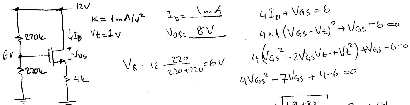
$$V_{GS1} = \frac{7 + \sqrt{49 + 32}}{8} = 2 \text{ V} \quad \text{valid}$$
