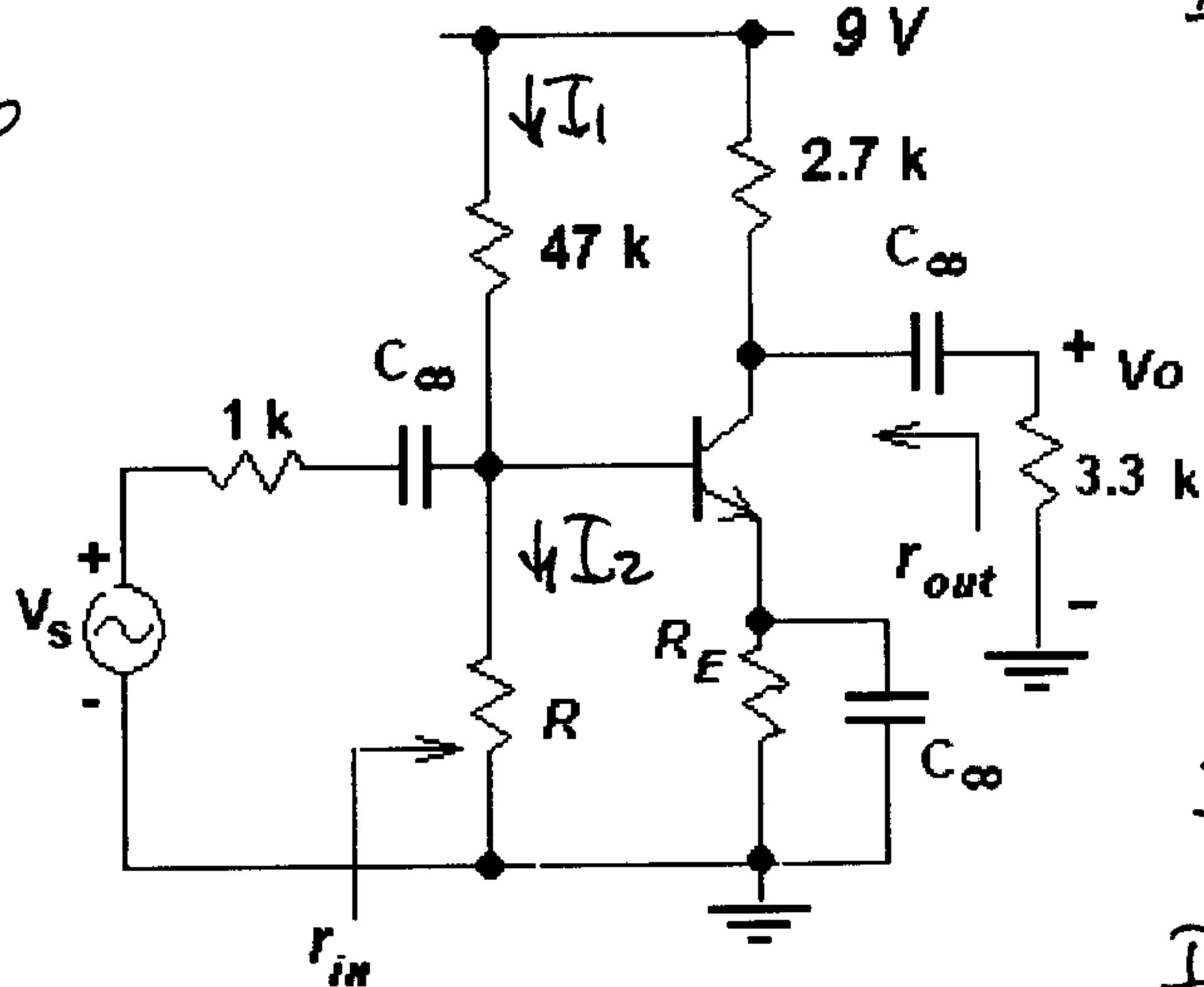
$$I_c \approx I_E \quad (R_E + R_C)I_c + V_{CE} = 9 \text{ V}$$
