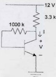
$$V_{BE} + I_B(1000 + 3.3(\beta+1))I_B = 12$$
