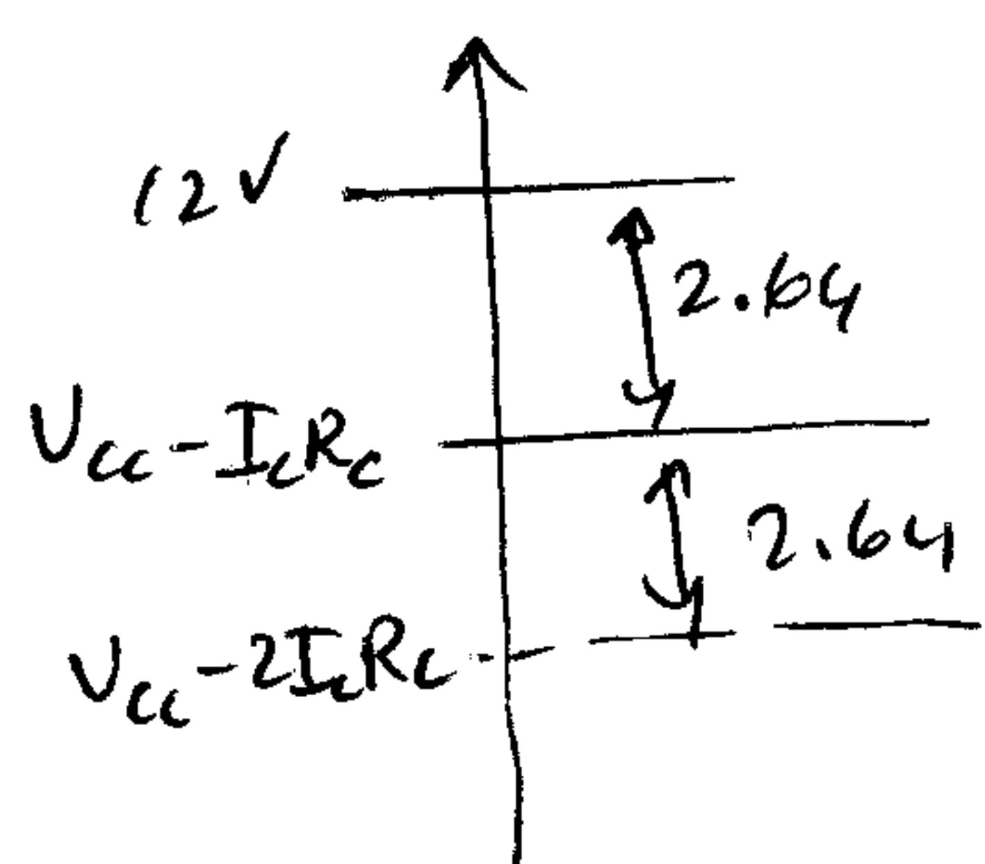
$$|v_{idm}|_{max} = \frac{2.64}{52.8} = 0.05 \text{ V}$$
