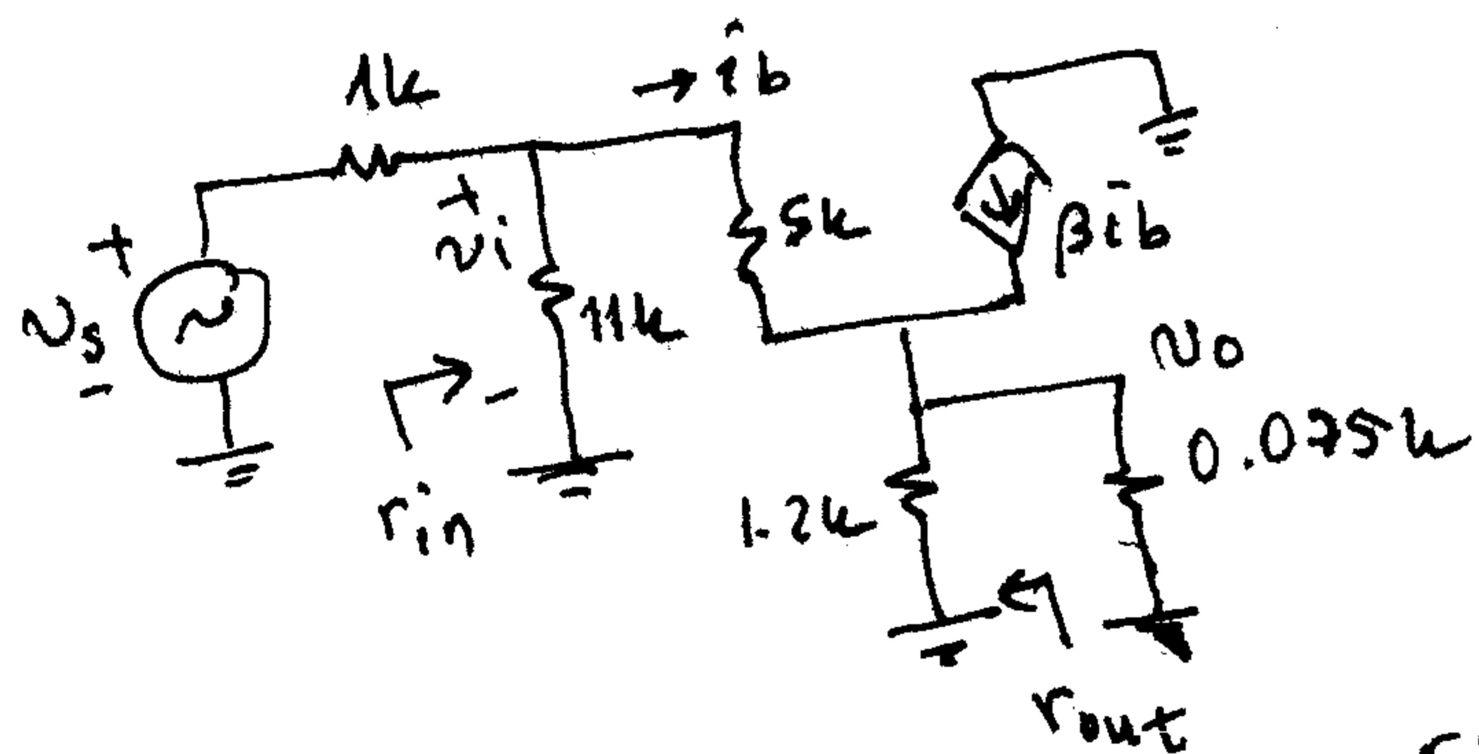
$$\frac{v_o}{v_i} = \frac{(\beta+1)(1.2 \parallel 0.075)}{r_{\pi} + (\beta+1)(1.2 \parallel 0.075)} = \frac{301 \times 0.07}{5 + 301 \times 0.07} = 0.808$$
