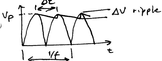
$$I = C \frac{\Delta V}{\Delta t} \rightarrow \Delta V = \frac{I \Delta t}{C} = \frac{0.4 \times \frac{1}{100}}{1000 \times 10^{-6}} = 4 \text{ V}$$
