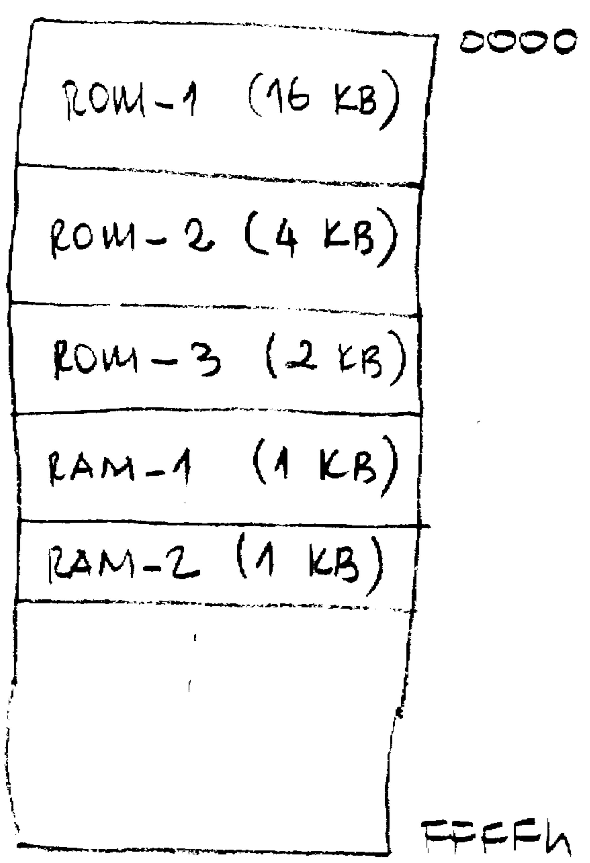
In a 8085 based microprocessor system, 22 KByte ROM, 2 KByte RAM memory is needed. Locations of memory ICs are shown in the memory map shown in the figure.
