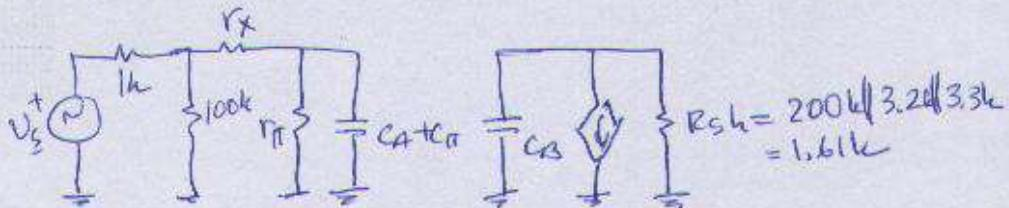
$$C_{\pi} = \frac{g_m}{2\pi f_T} - C_{\mu} = \frac{48 \times 10^3}{2\pi \times 200 \times 10^6} - 2 \times 10^{-12} = 3.62 \times 10^{-12} \text{ F}$$
