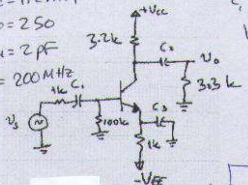
$$C_1 = C_2 = C_3 = 100 \text{ pF}$$
