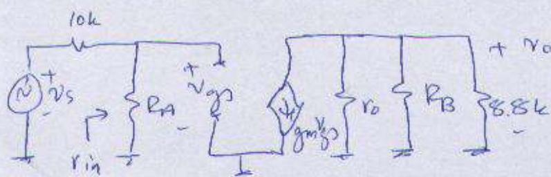
$$R_{sh} = r_o \parallel R_B \parallel 8.8k$$
