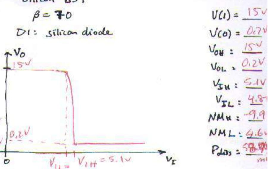
$$Q: OFF, V_o = V(1) = V_{OH} = 15V$$
