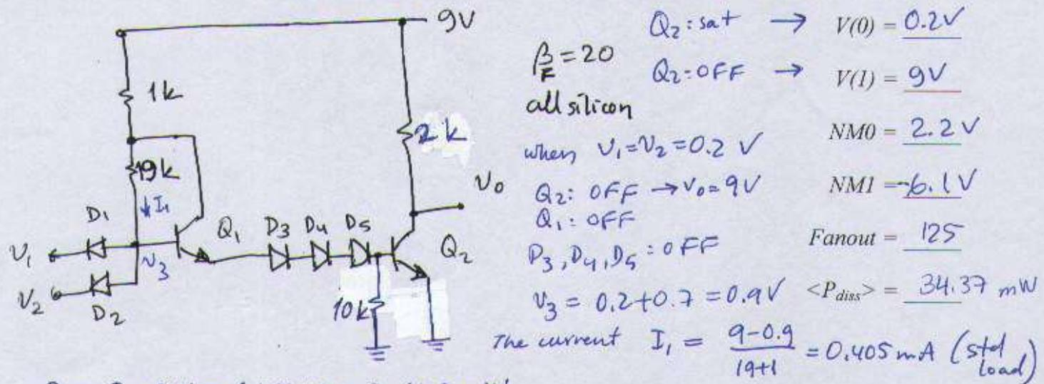
$$P_1 = I_1 \times 9V = 0.405 \times 9 = 3.645 \text{ mW}$$
