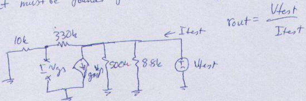
$$r_{out} = \frac{V_{test}}{I_{test}}$$
