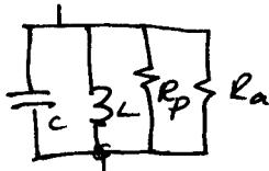
$$Q = \frac{R_p}{\omega_0 L} \rightarrow R_p = Q \omega_0 L = 200 \times 2\pi \times 10^6 \times 10 \times 10^{-6} \Omega \quad R_p = 12566 \Omega$$
