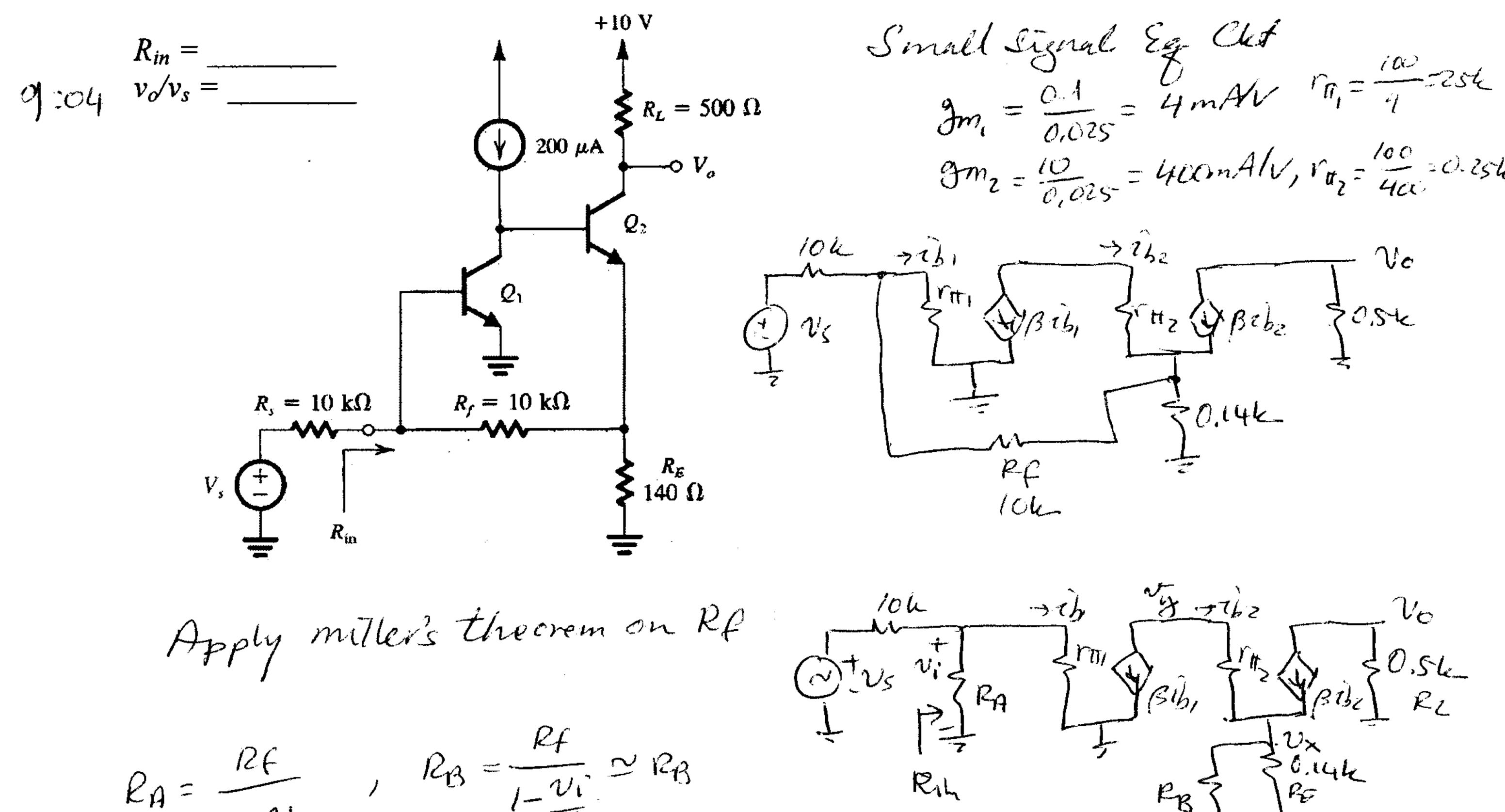
$$\frac{V_{i}}{V_{i}} = \frac{V_{i}}{V_{j}}, \quad \frac{V_{i}}{V_{i}} = \frac{(\beta+i)(R_{\beta}/R_{e})}{r_{\pi_{1}} + (\beta+i)(R_{n}/R_{e})} = \frac{101 \times 0.14}{0.15 + 101 \times 0.14} = 0.9826$$
