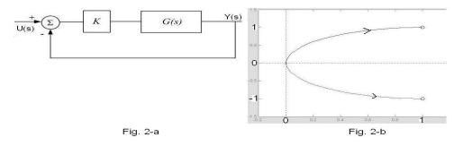
2. [33 pts.] Consider the configuration in Fig. 2-a. Determine a transfer function G(s) such that the pole locations of the closed-loop transfer function  $\frac{Y(s)}{U(s)}$  are as shown in Fig. 2-b as K changes from 0 to infinity. **Ans.** This graphics occurs if there are zeros at 1 + i and 1 - i, and there are two poles at the origin. Thus  $G(s) = \frac{(s-1+i)(s-1-i)}{s^2} = \frac{s^2-2s+2}{s^2}$
