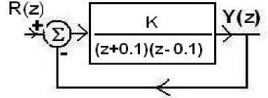
(a)  $\frac{K}{z^2+K-0.01}$ (b) For  $K \ge 1.01$  the system is unstable. (c) Because the system is stable for K = 0.5, we have  $y(\infty) = \lim_{z \to 1} (z-1) \frac{z}{z-1} \frac{0.5}{z^2+0.5-0.01} = \frac{0.5}{1.49} = 0.3356$
