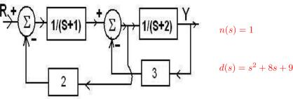
**2.** For the figure below, sketch the root locus. Find all positive K values that make the closed loop system unstable.
