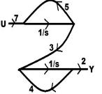
25 pts. Given the LTI systems with their transfer functions on the left write the transfer function  $\frac{Y(s)}{U(s)}$ .
