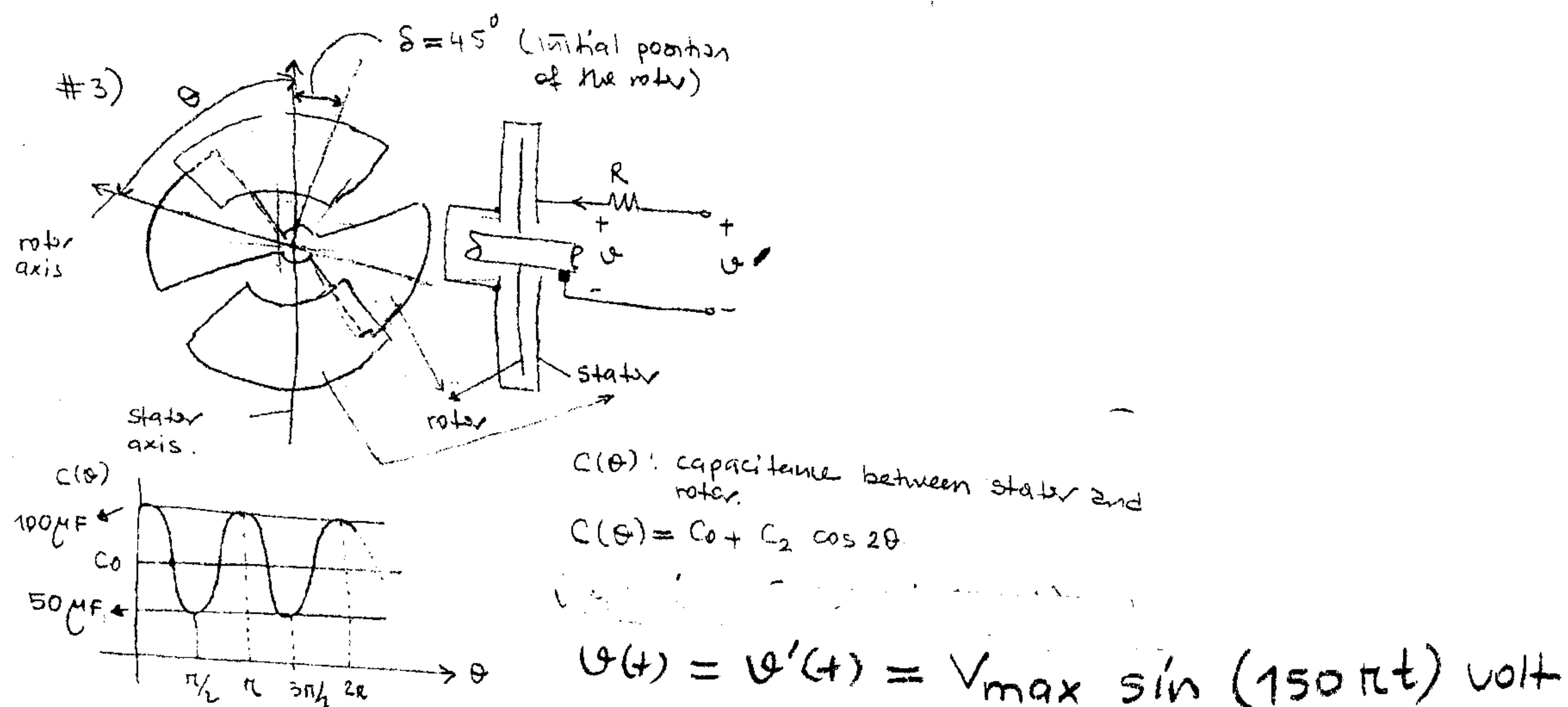
Consider the electrostatic motor given in the above.
