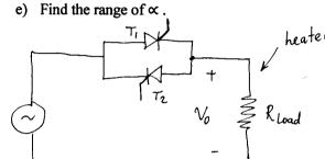
b) There are two thyristors connected back-to-back. Also a controller responsible from generating the proper triggering pulses to the thuristors.
