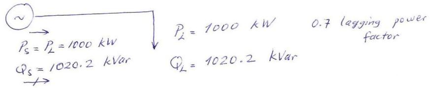
a) if a shunt capacitor is connected to the system,
