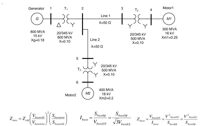
(b) (15): The motors  $M_1$  and  $M_2$  in the problem 1 are drawing their rated powers from the system at the rated terminal voltages. In addition, the both motors are operating at 0.8 lagging power factor. Find the current supplied by the generator in per-unit and in Amperes.
