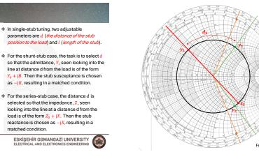
Shunt-Stub For a load impedance  $Z_L = 60 - j80 \Omega$ , design two single-stub Example (short circuit) shunt tuning networks to match this load to a  $50 \Omega$  line.  $z_L = 1.2 - j1.6$  $y_L = 0.3 + j0.4$  $y_1 = 1.0 + j1.47$  $d_1 = 0.110\lambda$
