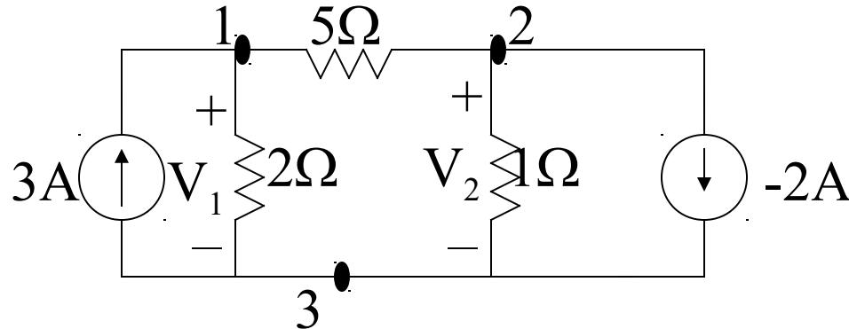
Consider the circuit with 3 nodes. Select one of the nodes as the reference node and assign voltages to two remaining nodes as  $V_1$  and  $V_2$ .
