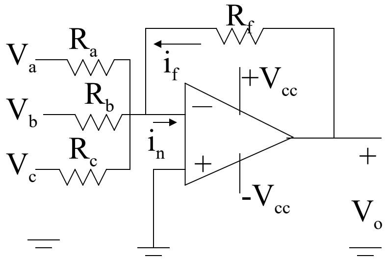
$$\begin{aligned} V_p &= V_n = 0 & i_n &= 0 \\ \frac{-V_a}{R_a} + \frac{-V_b}{R_b} + \frac{-V_c}{R_c} + \frac{-V_o}{R_f} &= 0 \\ V_o &= -\left( \frac{R_f}{R_a} V_a + \frac{R_f}{R_b} V_b + \frac{R_f}{R_c} V_c \right) \end{aligned}$$
