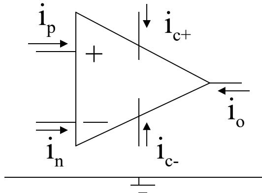
The equivalent resistance seen by the input terminals of the op amp is very large, typically  $1M\Omega$  or more. Ideally, the input resistance is infinite, resulting in the current constraint  $i_p = i_n = 0$ .
