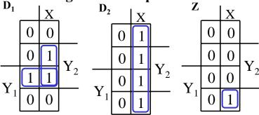
$\mathbf{D}_1 = \mathbf{Y}_1 \mathbf{Y}_2 + \mathbf{X} \overline{\mathbf{Y}}_2$ **Gate Input Cost = 9** Select this state assignment for  $D_2 = X$
