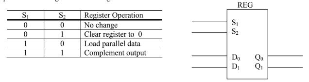
Use JK flip-flops in the register. Use only the inputs J and K to perform the listed operation. (20 pts)
