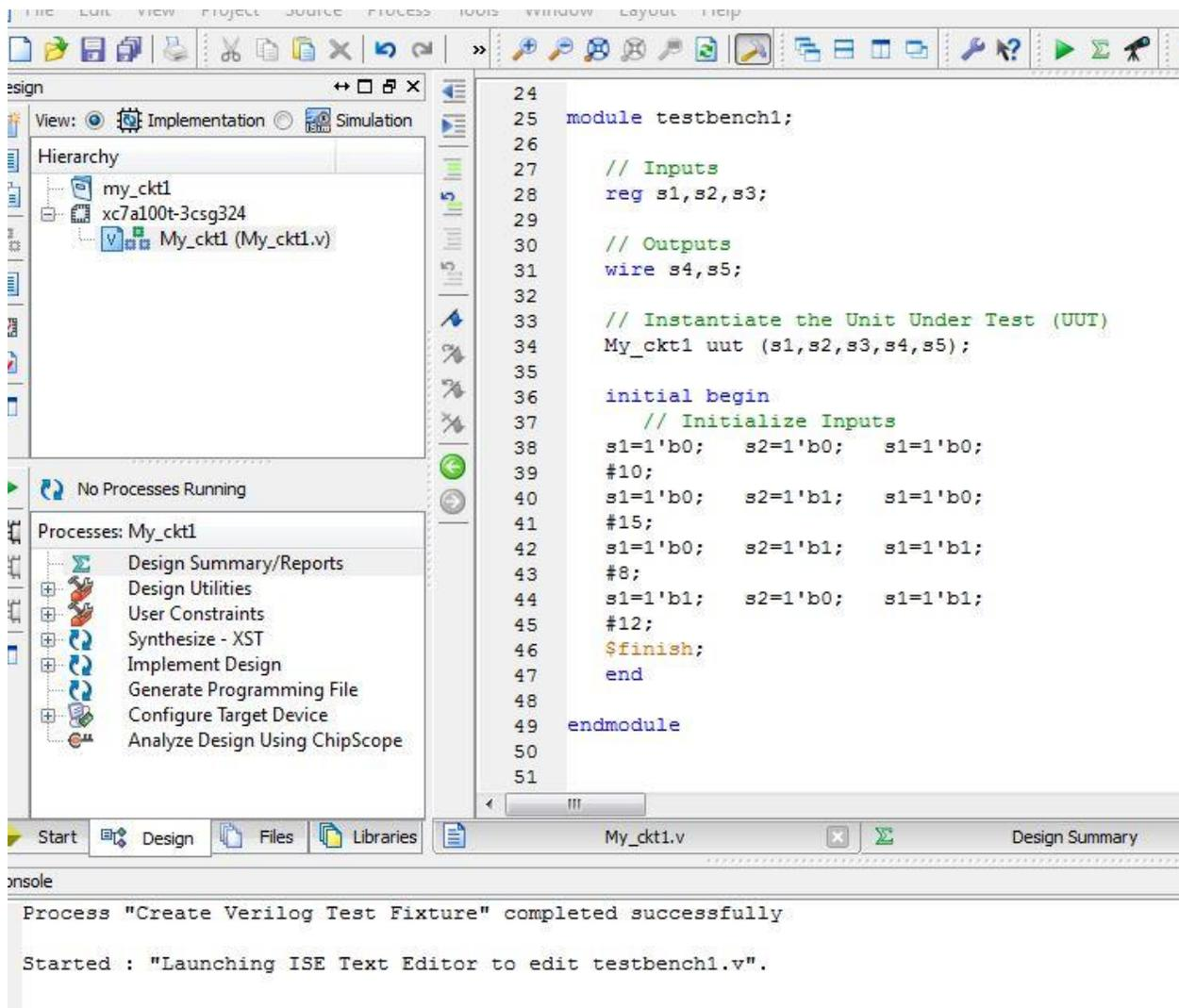
**Figure 8:** Completed Test bench
