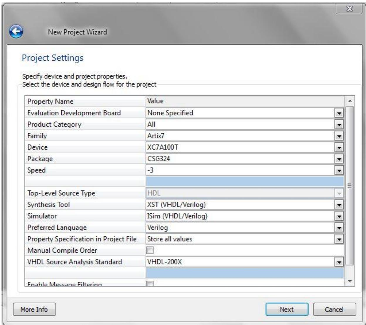
**Figure 2:** New Project Wizard - Device Properties
