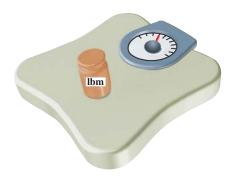
FIGURE 1–16 A mass of 1 lbm weighs 1 lbf on earth.
