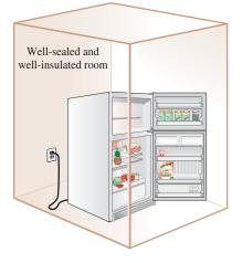
A refrigerator operating with its door open in a well-sealed and well-insulated room.
