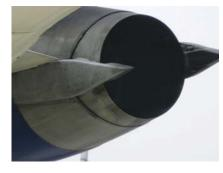
In jet engines, the high-temperature and high-pressure gases leaving the turbine are accelerated in a nozzle to provide thrust.
