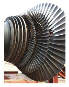
FIGURE 5–29 Turbine blades attached to the turbine shaft. ©Miss Kanithar Aiumla-Or/Shutterstock RF
