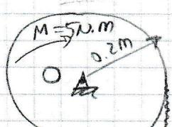
$$\begin{aligned}m &= 30 \text{ kg} \\ \omega_0 &= 0 \\ \omega &= 20 \text{ rad/s} \\ \theta &= ? \\ O_x &=? \quad O_y = ? \\ F &= 10 \text{ N} \\ M &= 5 \text{ N.m}\end{aligned}$$
