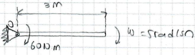
$$\begin{aligned} m &= 20 \text{ kg} \\ \omega &= 5 \text{ rad/s} \\ \alpha &=? \\ \alpha_x &=? \\ \alpha_y &=? \end{aligned}$$
