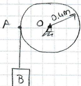
$$m_V = 60 \text{ kg} \\ r_0 = 0,75 \text{ m} \\ m_B = 20 \text{ kg} \\ \omega_B = 0 \\ \alpha = ?$$
