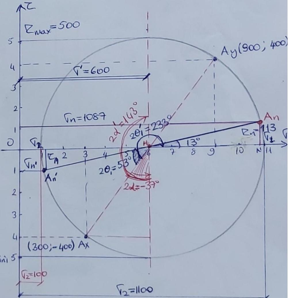
$$\tan 2\theta_i = \frac{4}{3} = \frac{2\Sigma_{xy}}{\Gamma_x - \Gamma_y} = \frac{2(-400)}{300 - 900} = \frac{800}{600} = \frac{4}{3} \Rightarrow (2\theta_i = +53^\circ \rightarrow \Gamma_2 = 100 \text{ N/cm}^2)$$
